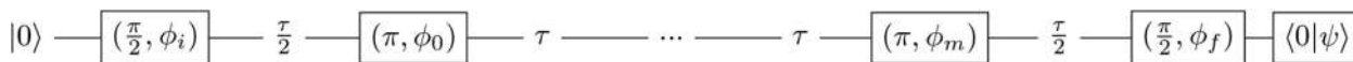
FIG. 23. Pulse sequence for Gauss sum factorization. A \pi/2 -pulse phase shifted by \pi/2 is used to rotate the qubit to the superposition state. Next, a train of m \pi -pulses is applied to the qubit. The phase of the first \pi -pulse is 0 and that of the k -th pulse is (-1)^k \pi(2k - 1)N/l where N is the number to factorize and l is the trial factor. Finally, a \pi/2 -pulse phase shifted by \pi/2 is used to rotate the system back to the computational basis. If l is a factor of N , the phase will be an integer number of \pi and the \pi -pulse train will be in phase, causing the final \pi/2 rotation to rotate the system to |1\rangle . Otherwise, an arbitrary rotation of the system will occur. The sequence is repeated for m from 1 to M , where M is the total number of pulses to be used, and the results are averaged by M . This is to reduce the impact of arbitrary non-factor rotations that may end up near |1\rangle . A delay \tau is applied between pulses.
