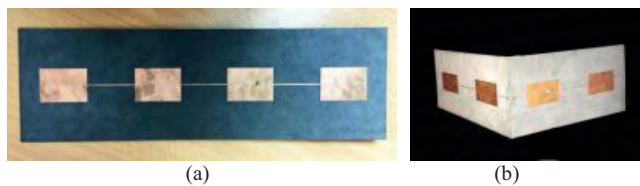
Fig. 20. Fabricated antennas: (a) Patch array with serial feed-line, and (b) convex bent array.
