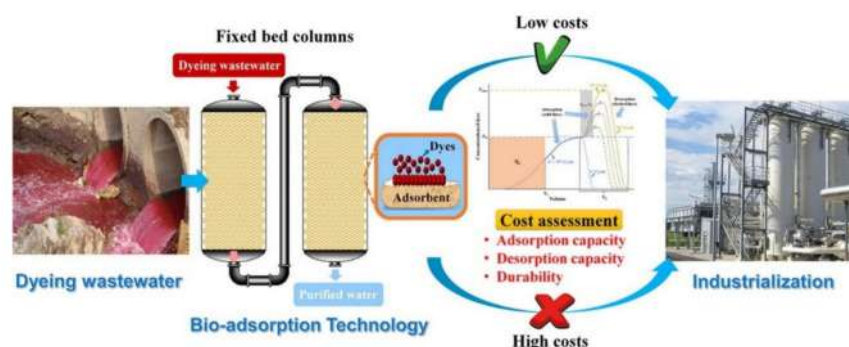
Figure 6. Adsorption of dyeing wastewater [85], with permission from Elsevier.
