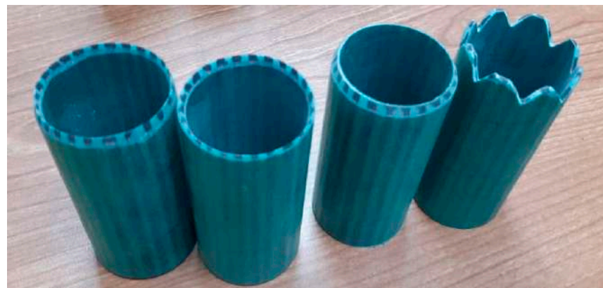
Figure 4. The different chamfered samples as the trigger mechanism.
