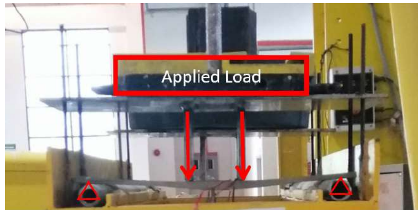
Figure 4. A coupon sample under four-point bending creep.
