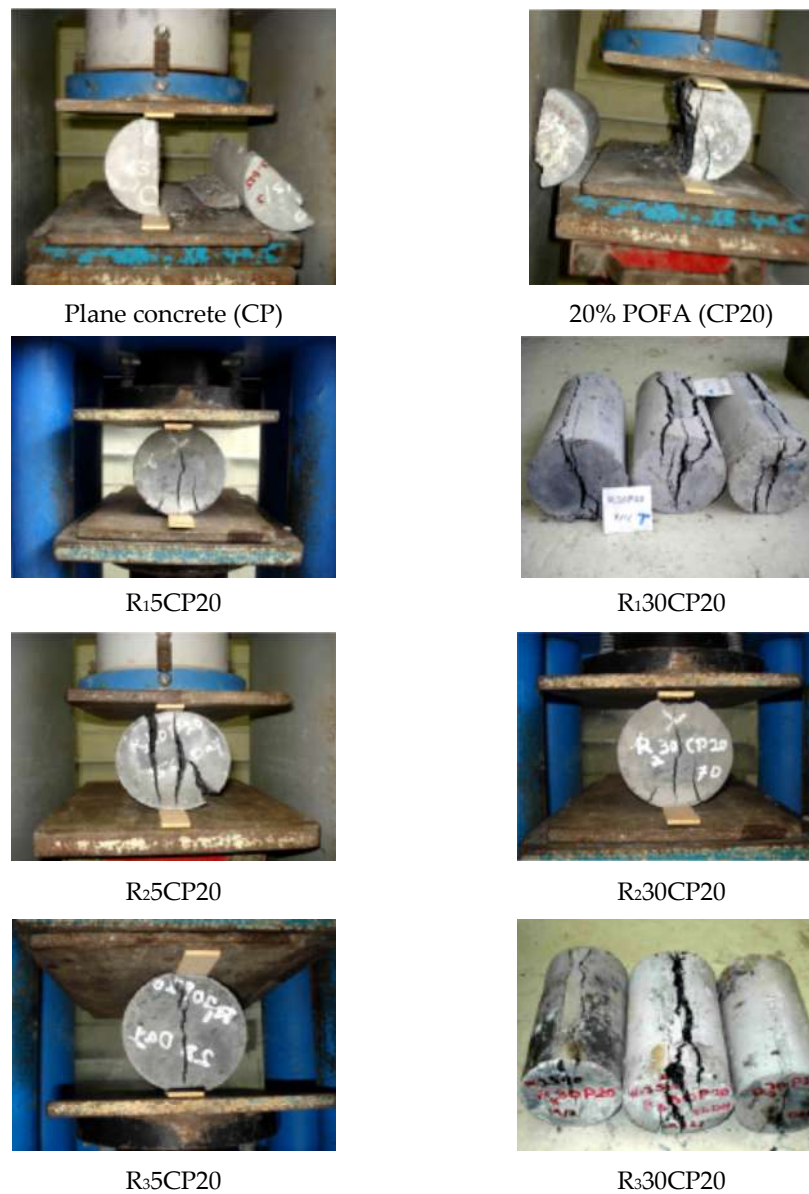
Figure 11. Rubberized concrete sample showing large deformation without disintegration by increasing the level of rubber particles in mixture.
