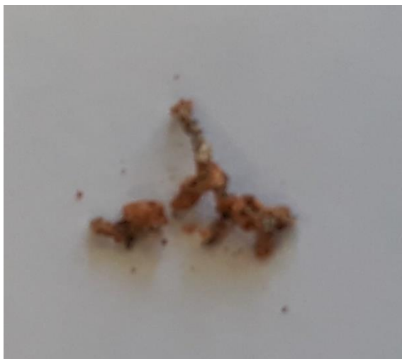
Figure 12. Fulgurite formation observed on sand after alternating high voltage testing.
