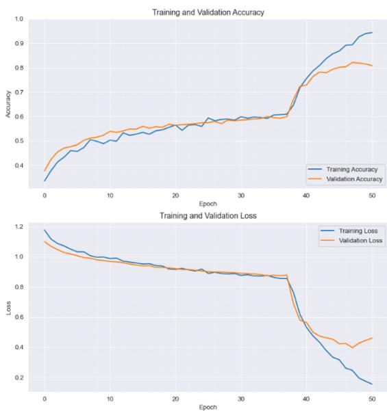
**Figure 6.** NasNet mobile training and validation accuracy and loss versus epochs for RGB image.
