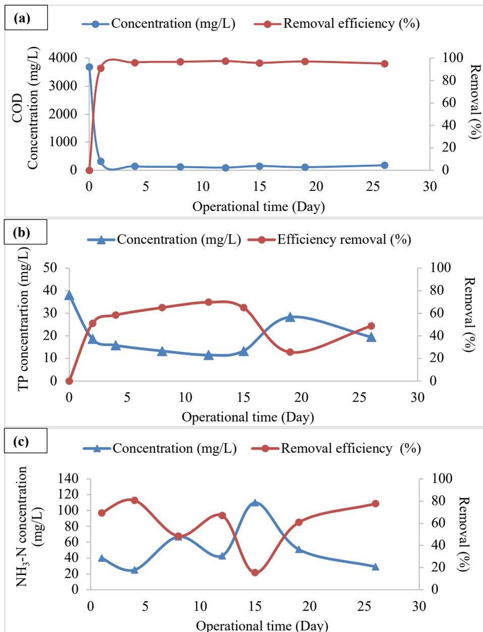
**Figure 4.** (a) COD concentration and percentage removal in PSBR system; (b) TP concentration of the effluent in PSBR; (c) Ammonia concentration of the effluent in PSBR; throughout 30 days experiment.
