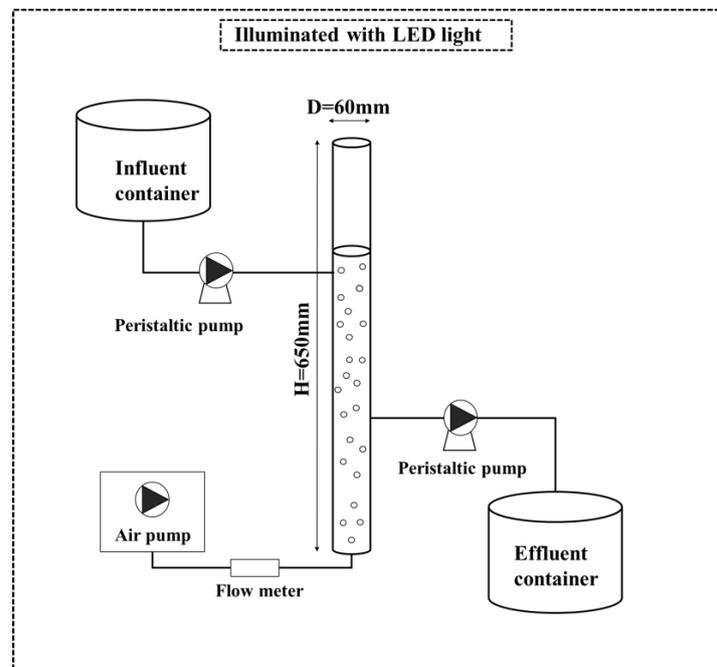
**Figure 1.** The simplified diagram of PSBR.
