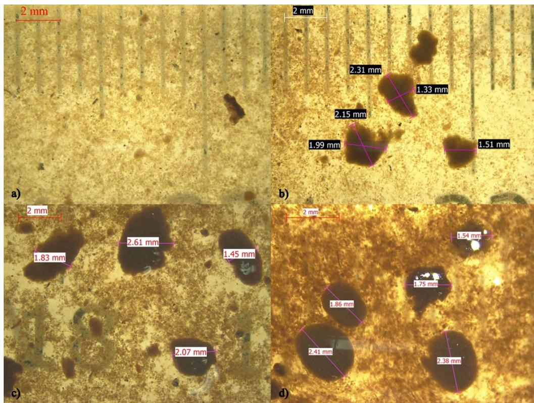
**Figure 2.** The development of microalgae-bacteria AGS inside the PSBR system **a)** Seed sludge; **b)** At 7<sup>th</sup> day of operation; **c)** At the 14<sup>th</sup> day of operation; and **d)** At 30<sup>th</sup> day of the experiment.
