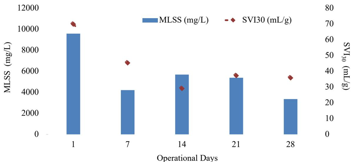
**Figure 3.** Dynamic of the biomass concentration (MLSS) and settle ability ( $SVI_{30}$ ) throughout the 30 days of experiment.
