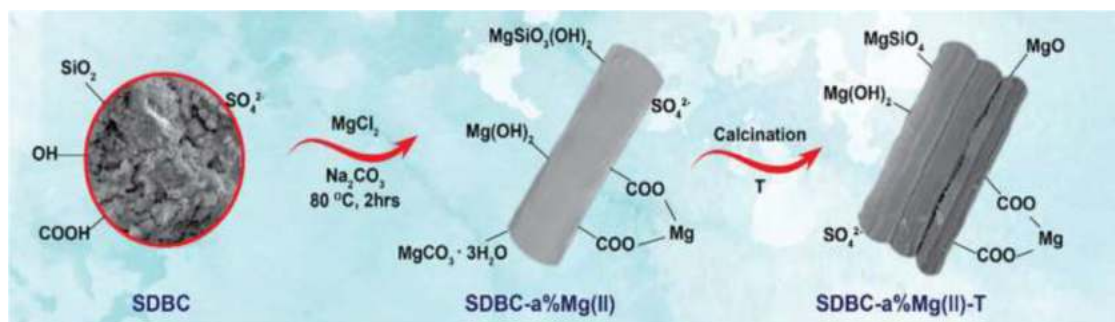
Fig. 12. Schematic illustration of the SDBC-a % Mg(II)-T synthesis and proposed morphological structure modifications retrieved from (Ngambia et al., 2019).
