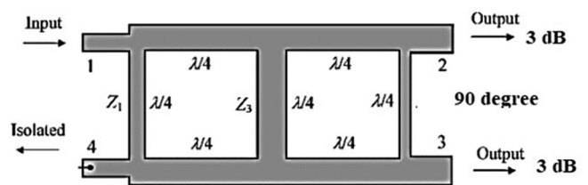
Fig. 1. General form of 3-dB hybrid coupler [14].
