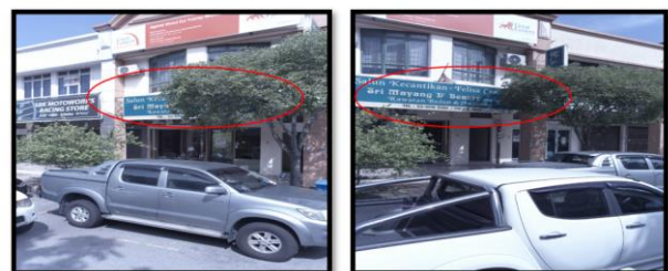
Figure 12. Example of blockers/noises for the building façade texture from raw 360 side cameras.
