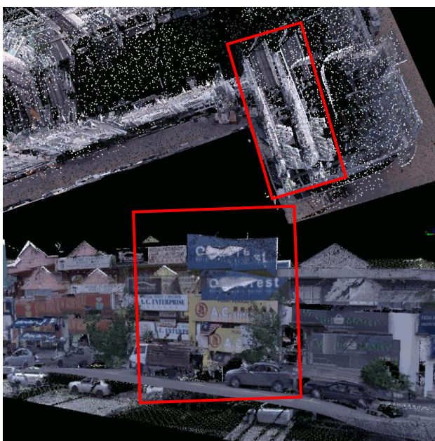
Figure 9. Example of MLS error - duplicate point clouds data of the same building with an axis shifted. They have potentially accrued in pre-processing of raw data duplicated moved as manual correction toward GCP.
