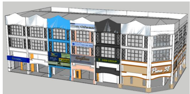
Figure 25. An example of correct geometry (splitted by lot), scale unique ID and .texture for each building unit.
