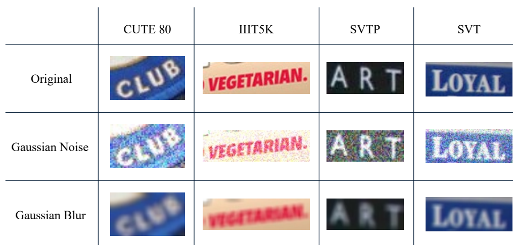
Figure 7. Sample images from the STR benchmarks processed by Gaussian blur and Gaussian noise. Gaussian noise of \sigma = 150 is added to the original image as noise processing, and a 3 \times 3 Gaussian kernel is convolved with the original image as blurring processing.
