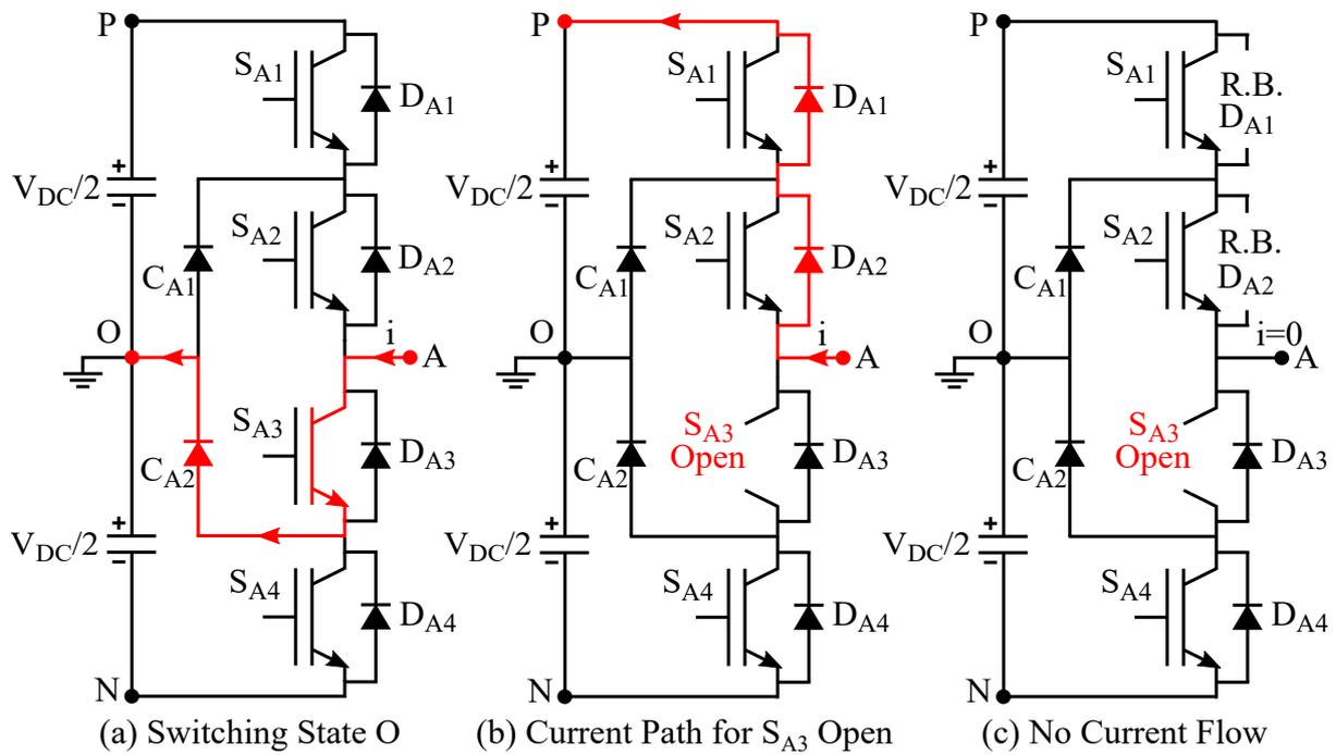
Figure 6. Circuit diagram for  $S_{A3}$  open switch fault.
