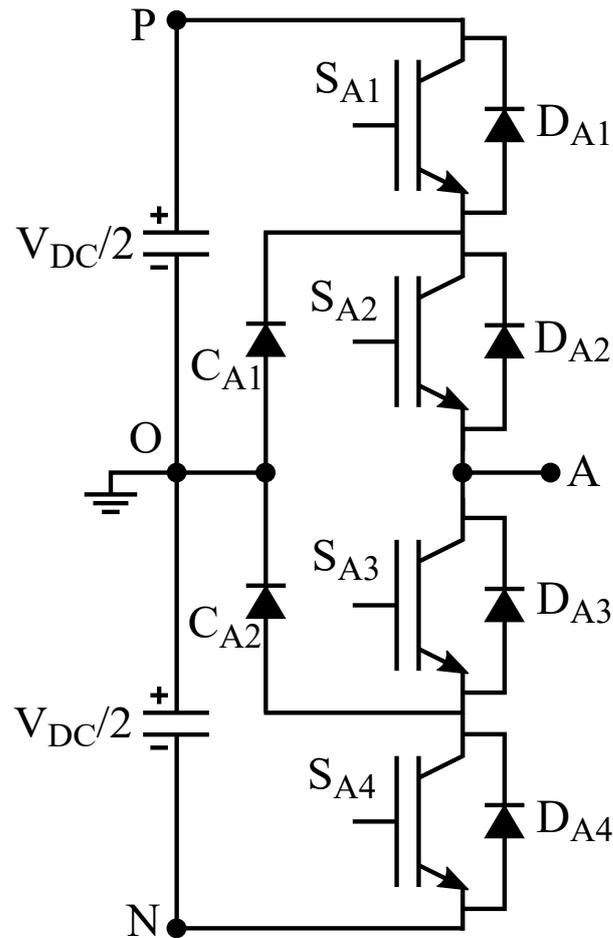
Figure 2. A leg of the NPC inverter.
