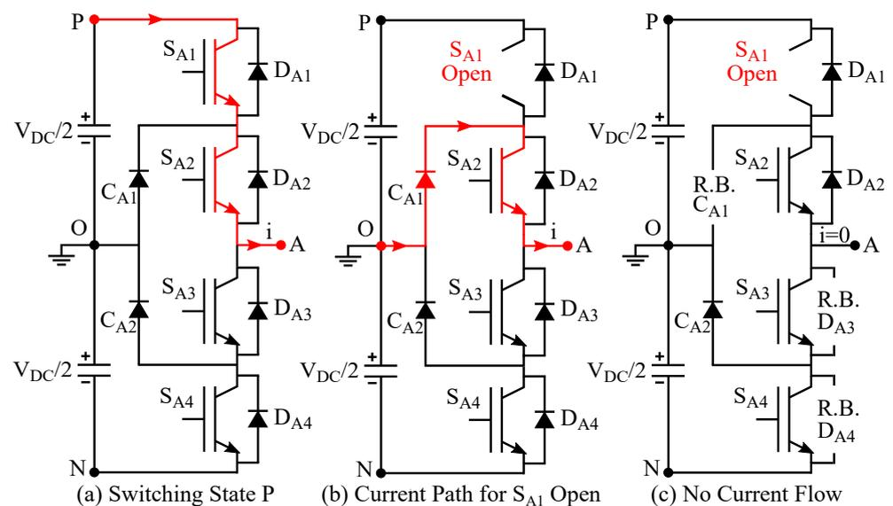
**Figure 4.** Circuit diagram for  $S_{A1}$  open switch fault.
