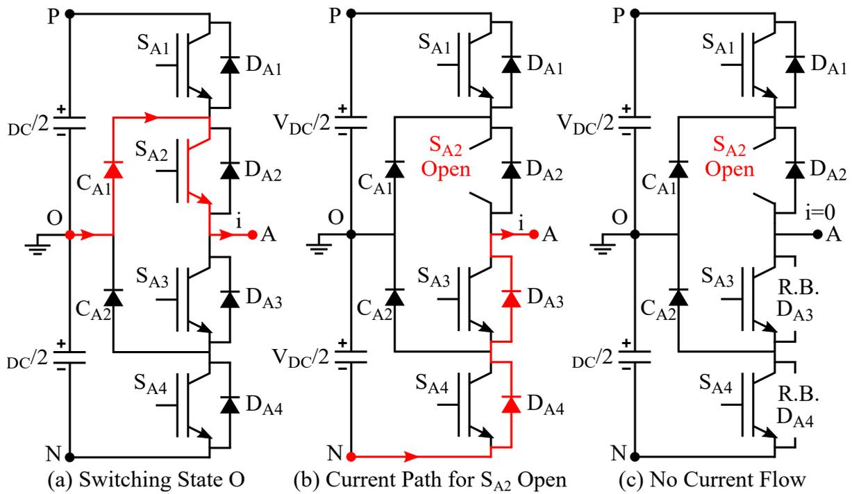
Figure 5. Circuit diagram for  $S_{A2}$  open switch fault.
