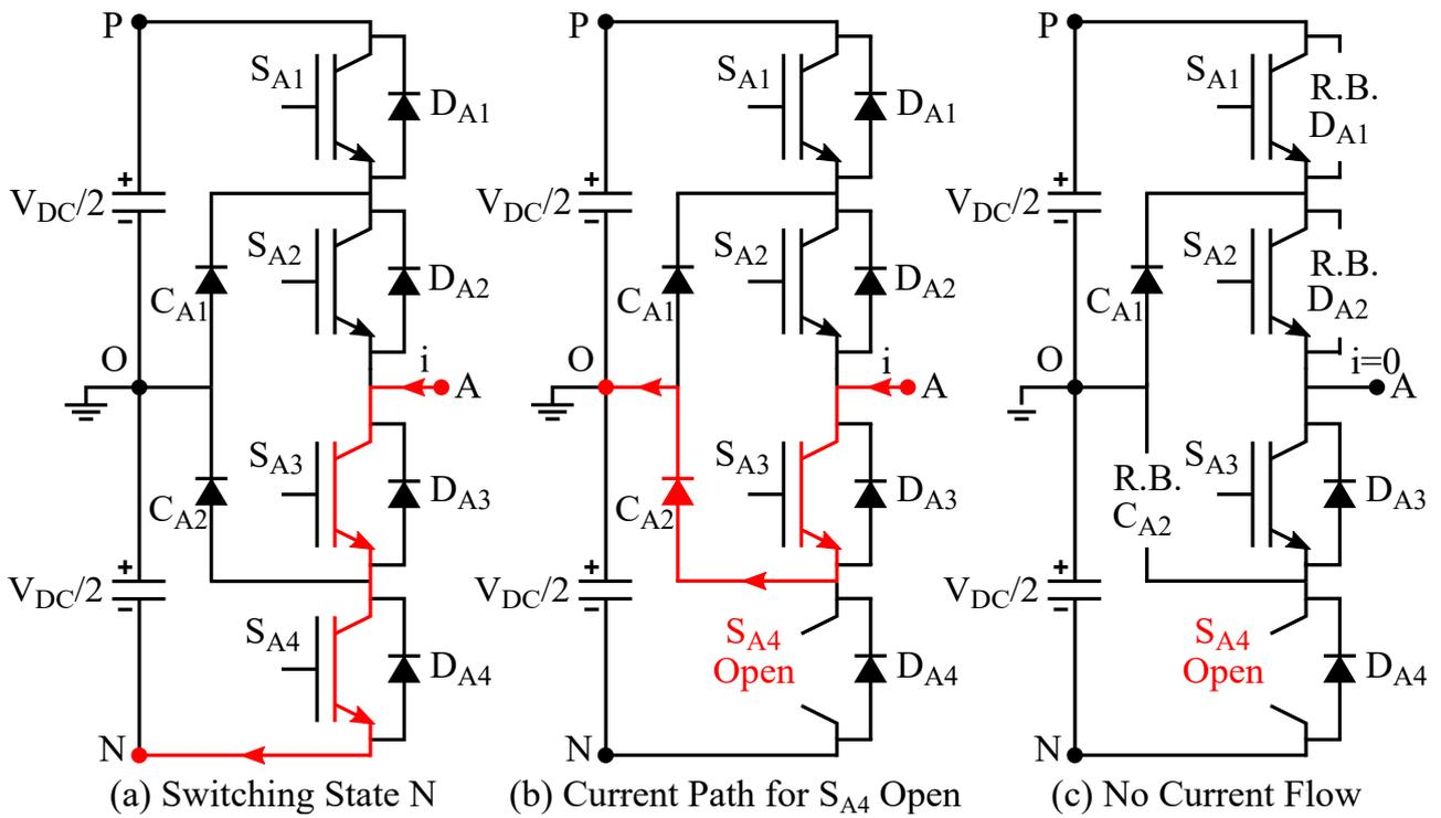
Figure 7. Circuit diagram for  $S_{A4}$  open switch fault.
