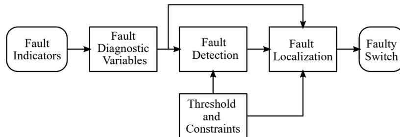
Figure 10. General schematic of fault diagnostic method.
