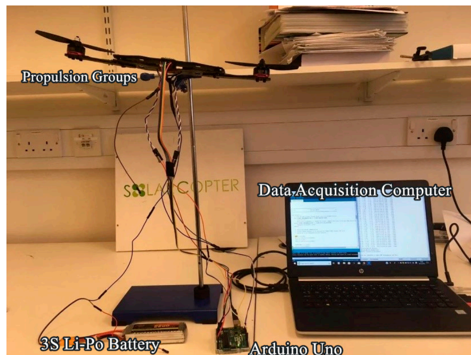
Figure 6. Two motors test bench.
