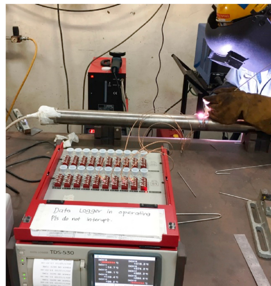
Fig. 2 – Welding process with thermocouples to record the transient temperature using the data logger.
