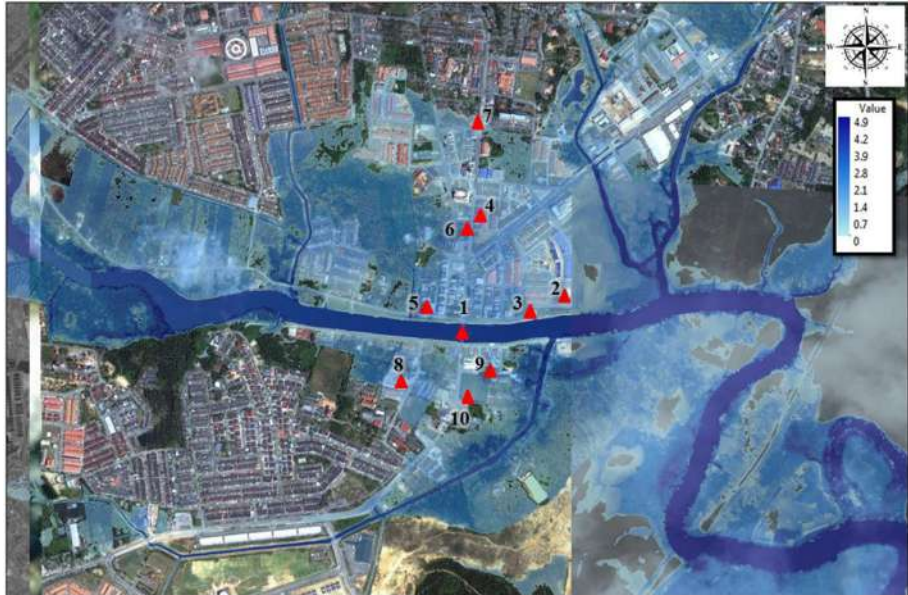
Fig. 15 The location of flood marks (triangle) for the 2007 flood event over the simulated flood coverage
