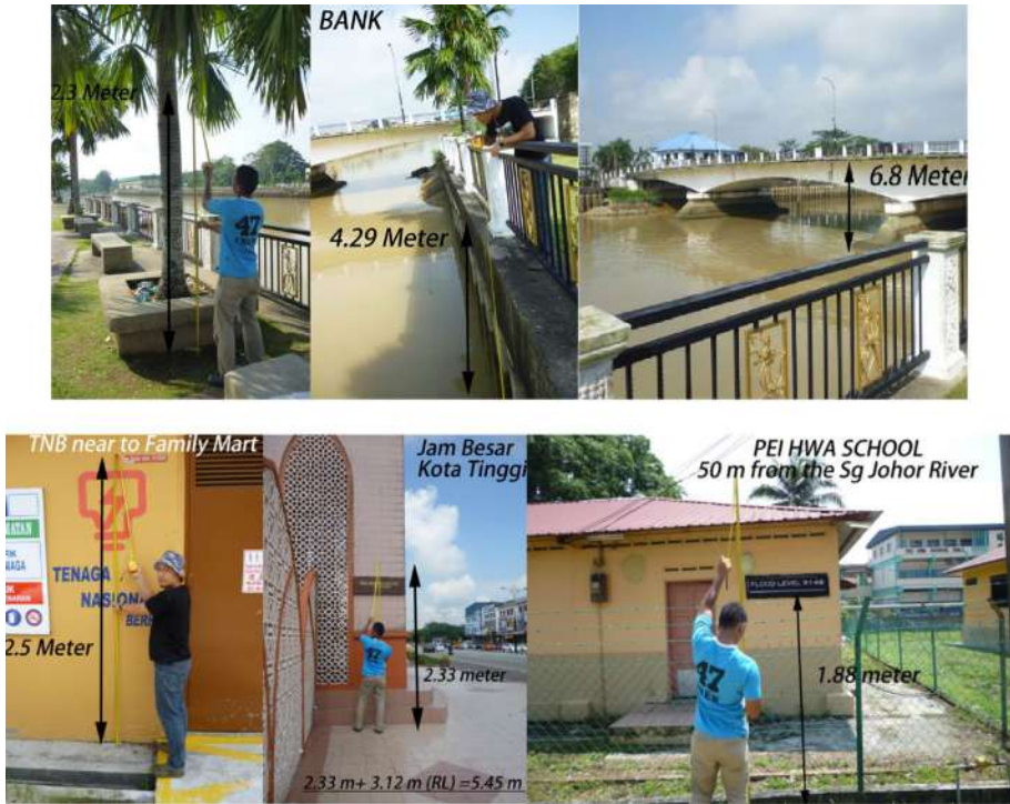
Fig. 8 Site verification on flood marks at the riverbank, bridge, and building at the flooded area in Kota Tinggi town
