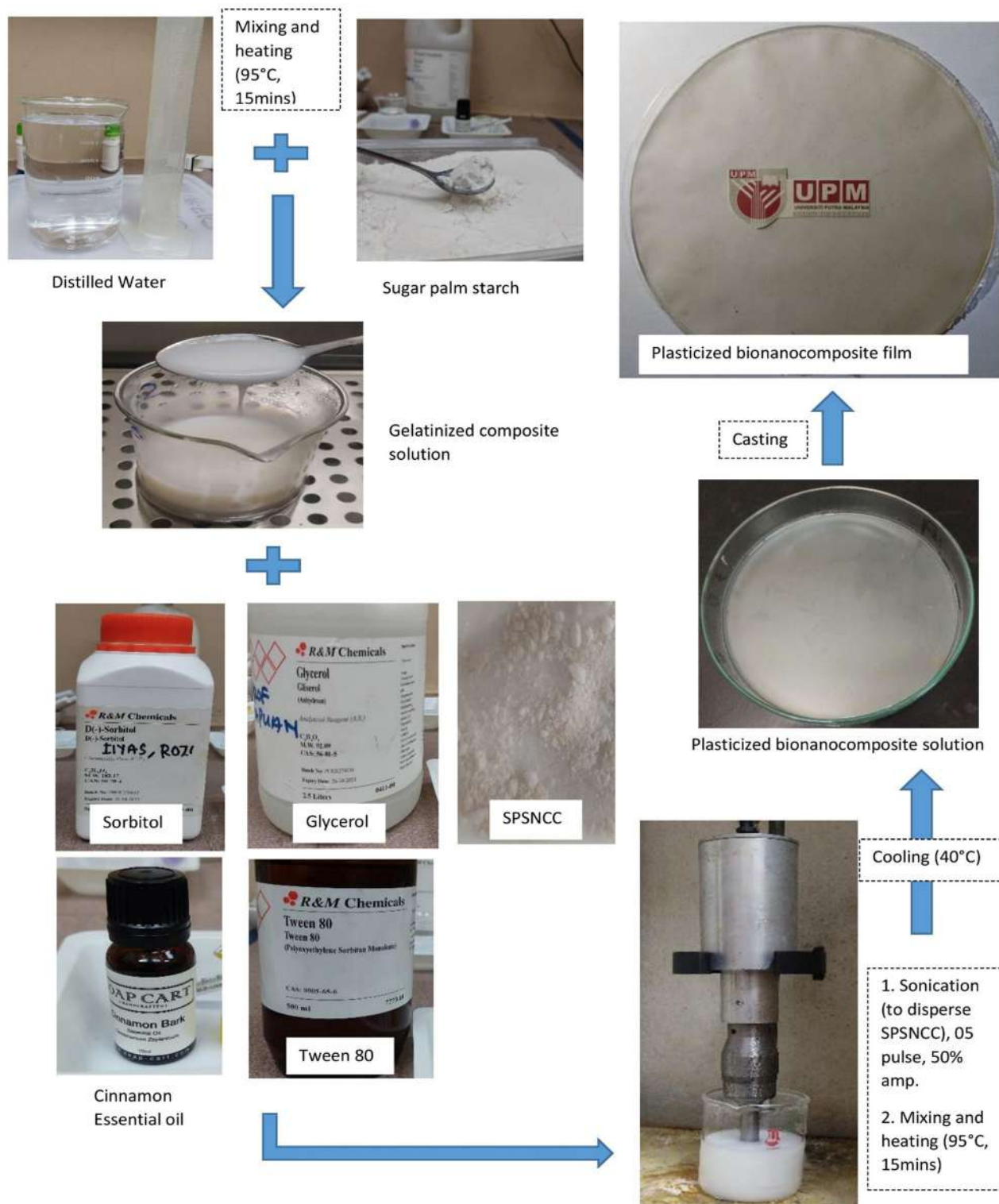
Figure 1: Processing flowchart of the bionanocomposite films.
