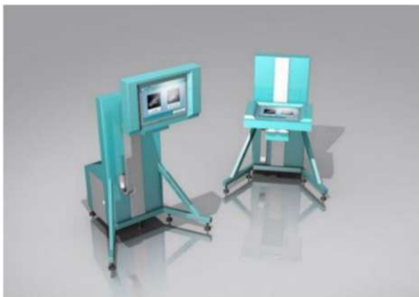
Fig. 8 CS WAVE [16]. The monitor is mounted on a specialised device, and the user can change its position to practice various welding techniques
