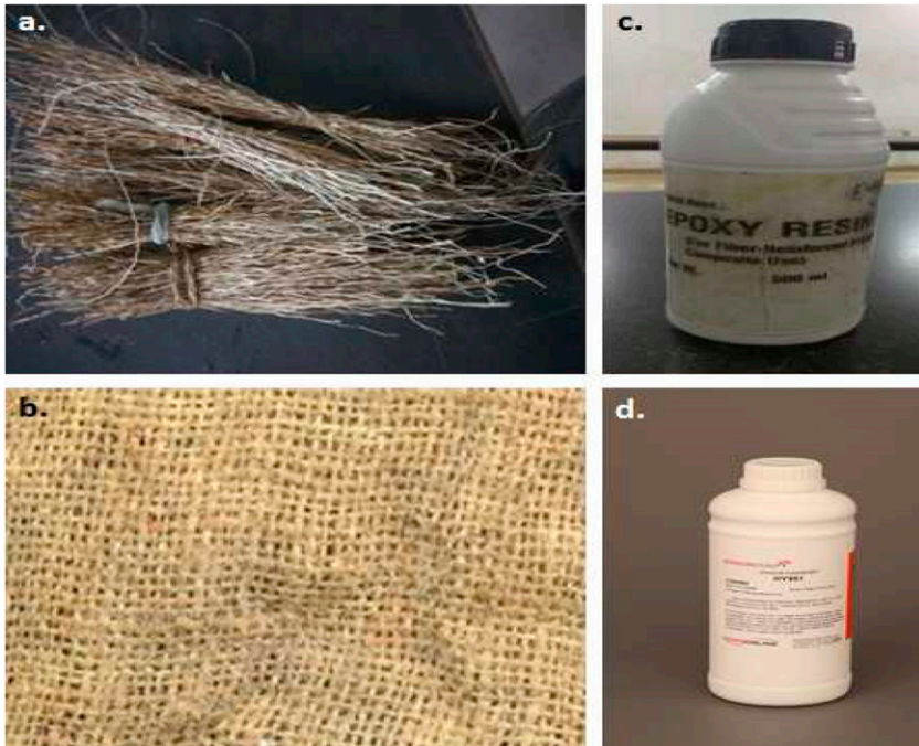
Figure 2. (a) Vetiver fiber, (b) jute fiber, (c) epoxy resin, and (d) hardener.
