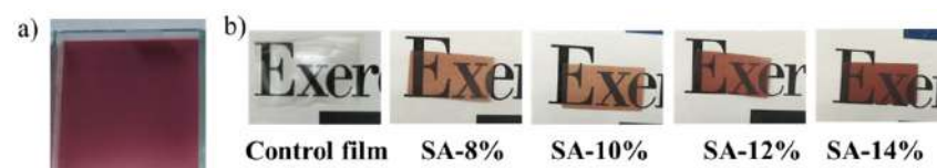
Figure 2. (a) The mixture solution cast into plate; (b) control film and RCA film physical appearance at four different concentrations.
