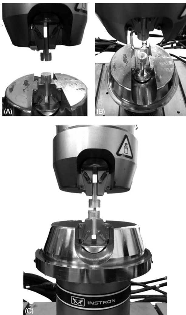
Fig. 4 A-C These photographs show the compression testing set-up. (A) In the mechanical testing process, compression platens were secured to the adjustable upper and lower grips of the Instron and (B) an allograft cortical bone cube was placed on the lower plate. (C) Axial force generated by the load cell compressed the specimen to failure.
