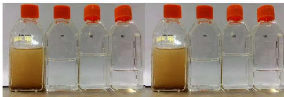
Figure 8. The visual result of change in color of lake water via non-treated and post-treated membrane after filtration.
