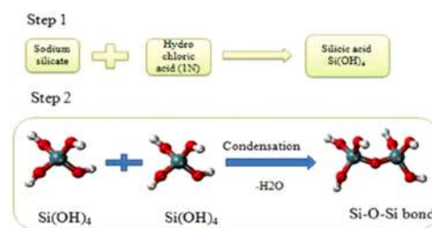
Fig. 7. Mechanism of silica particles formation from (a) coal fly ash [130]. Reprinted with permission from Springer Nature.
