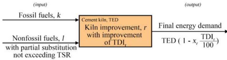
Fig. B.4 – Illustration of thermal energy constraint. k denotes fossil fuels, l denotes non-fossil fuels, r denotes kiln improvements, TED denotes the energy demand, TDI_r denotes the improvement by selected technologies r , and TSR denotes the substitution rate of non-fossil fuels l .
