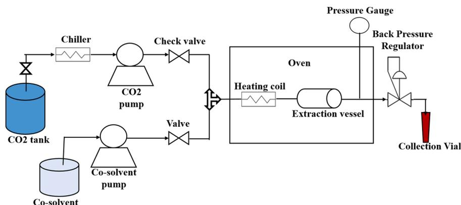
Fig. 1. SC-CO<sub>2</sub> schematic diagram at a CLEAR laboratory.
