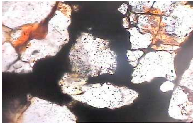
Figure 9. Photomicrograph of mix of nano-sized wet-ground cement and fine aggregates showing dense cement phase and good contact between cement paste and aggregate grains (magnification of 60× under non-polarized light).
