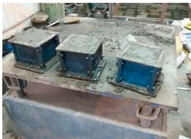
Figure 6. Concrete specimen in the mould on vibrating table.
