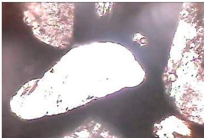
Figure 11. Photomicrograph of mix of nano-sized dry-ground cement and fine aggregates showing dense cement phase and good contact between cement paste and aggregate grains (magnification of 60× under polarized light).
