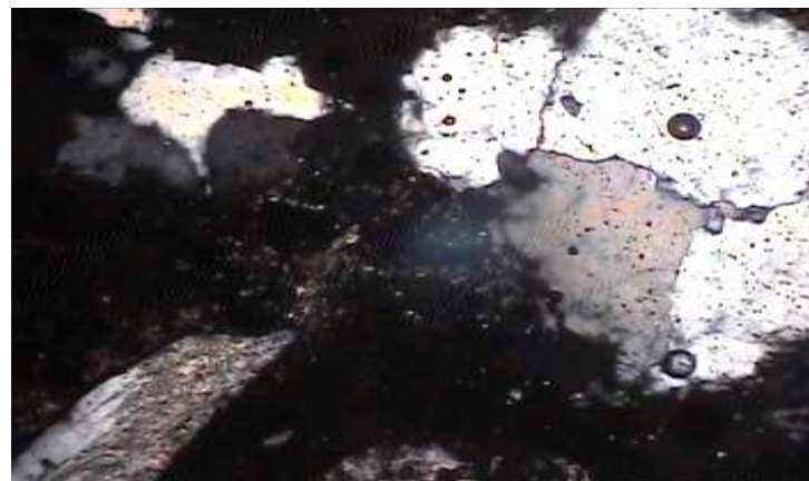
Figure 8. Photomicrograph of mix of nano-sized dry-ground cement and fine aggregates showing dense cement phase and good contact between cement paste and aggregate grains (magnification of 60× under non-polarized light).
