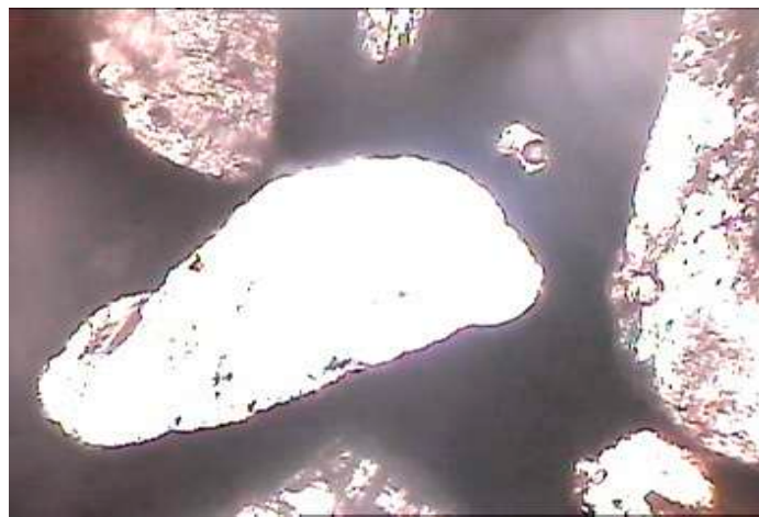
Figure 7. Photomicrograph of normal cement–fine-aggregate mix showing micropores within cement and loose contact between cement paste and aggregate grains (magnification of 60× under non-polarized light).
