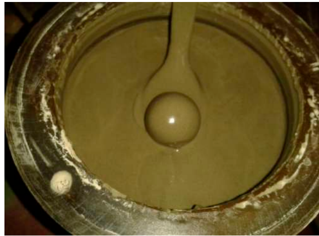
Figure 3. Inside view of wet-grinding of cement.
