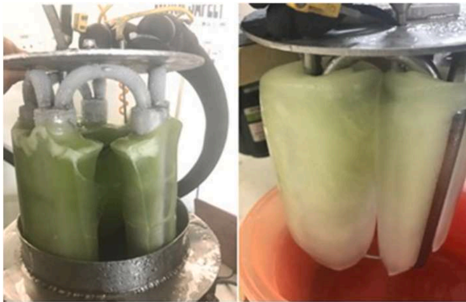
Fig. 5. An improvement of ice crystallization surface area using MPCC.
