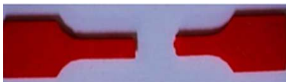
Figure 7. 3D printed ASTM D638 specimen after failure.
