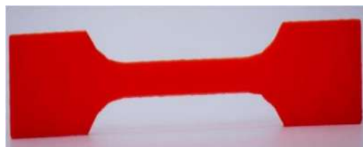
Figure 2. Test Specimen—ASTM D638.
