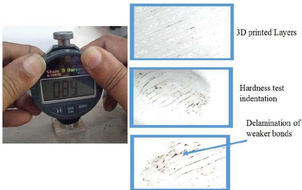
Figure 10. Hardness test setup and delamination of weaker bonds of 3D-printed test specimen.
