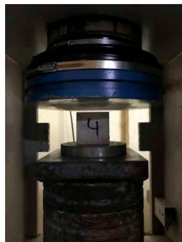
Figure 2. Mortar compression test.
