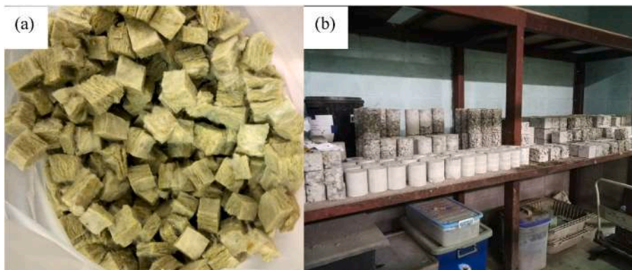
Fig. 1. (a). Rock wool in cubic shape; (b) air-dried curing environment.
