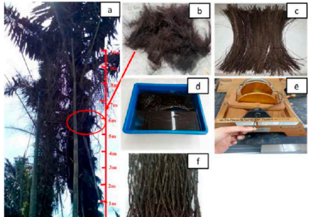
Figure 1. Preparation of SPF from sugar palm tree: (a) locating suitable SPF at the trunk, (b) SPF bundle, (c) combed SPF, (d) SPF treatment by alkalisation, (e) fibre yarning, and (f) finalised SPF yarn. Adapted with permission from Ref. [71]. Copyright Elsevier.
