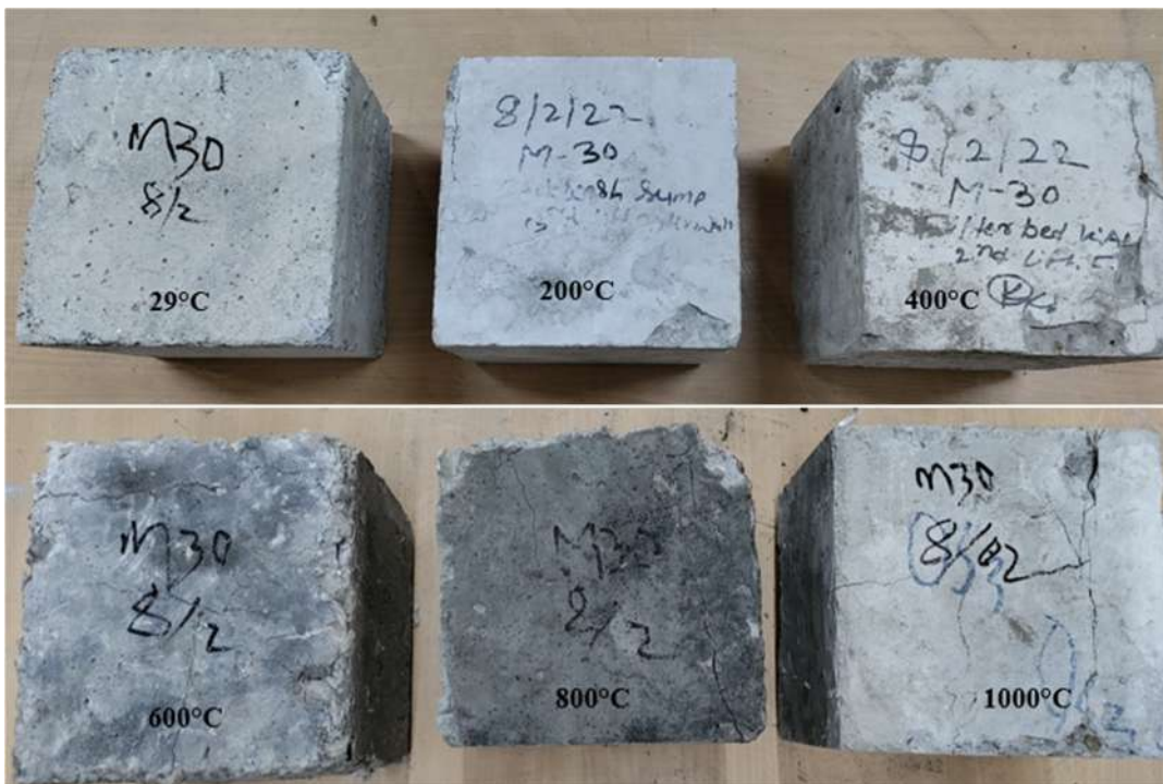
Figure 4. Concrete samples after elevated temperature.
