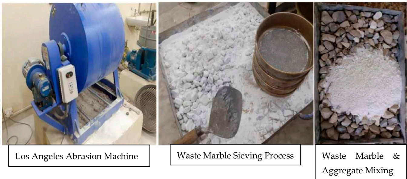
Figure 2. Mineral filler preparation.
