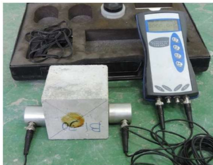
Figure 3. The ultrasonic pulse velocity test device.
