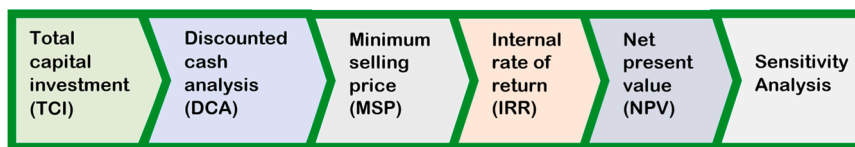
Fig. 4. Procedure for performing the sensitivity analysis and calculating net present value (NPV).
