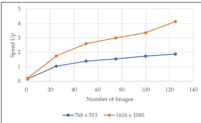
Figure 8: The GPU speedup for different number of image and image pixels for kernel 3.
