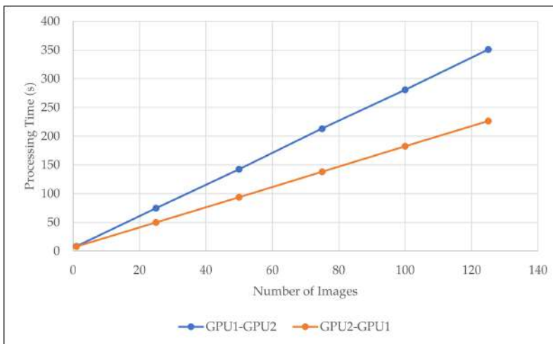
Figure 5: The processing time of two different architectures using two GPUs for different number of images for kernel 1 and kernel 2.
