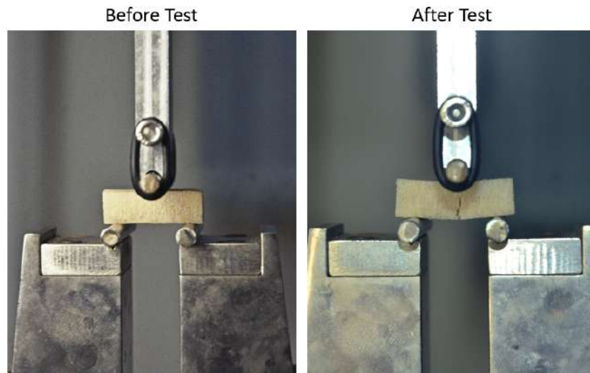
Fig. 2 The cancellous bone specimen before (left) and after test (right).
