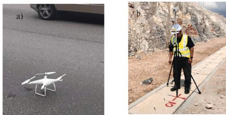
Fig. 3. UAV and GCP survey a) DJI Phantom 4 v2.0 UAV system b) SOUTH G1 GNSS system.
