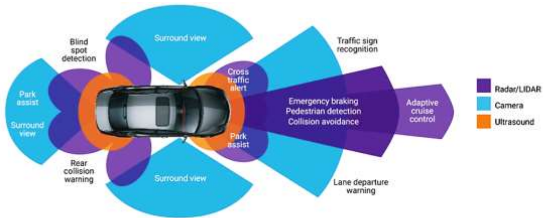
Figure 1.1 Sensors of ADAS [3]
