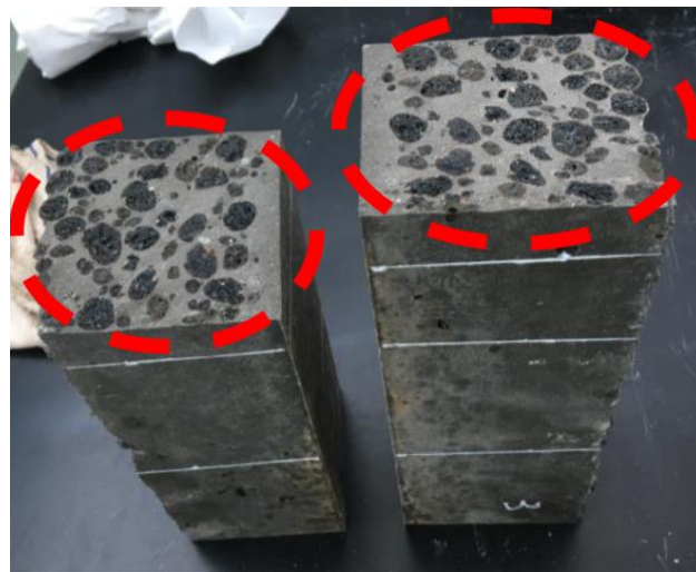
Figure 8 Centre-fracture of flexural specimens with fracture in aggregate
