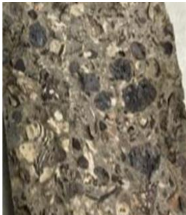
Figure 9 Shear failure of the OPS- and expanded clay-contained specimens
