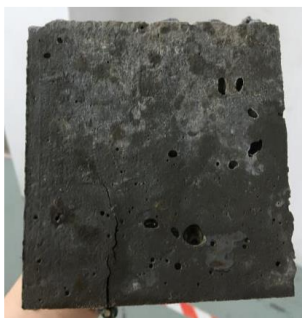
Figure 7 Shrinkage cracks of EC75-OPS25 at 28 days of curing age
