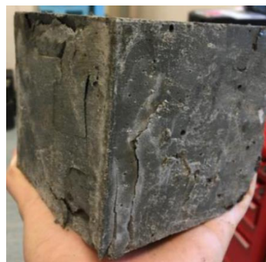
Figure 3 Cube failure under compressive load
