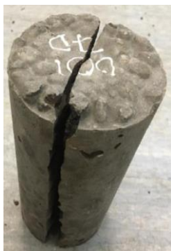
Figure 4 Failure mode of splitting tensile test specimen
