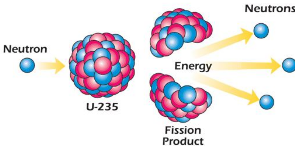
Figure 1.2 The formation of nuclear energy from the splitting of atoms (Department of Energy and Mineral Engineering, 2018)
