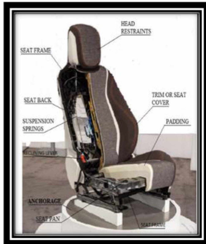
Figure 1.2 Cut section of driver seat components and systems (Kale and Dhamejani, 2015)
