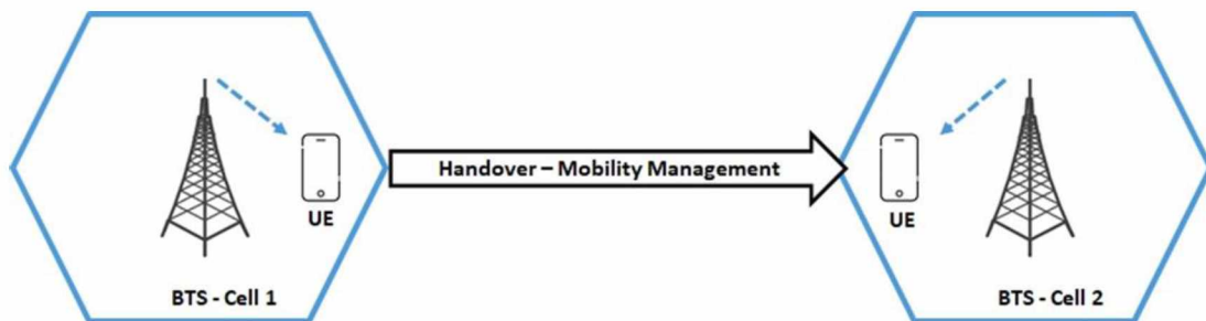
Figure 1. 1 UE Handover Between Two Cells
