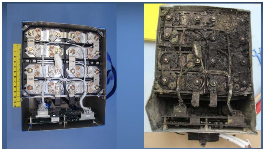
Figure 1.1 A new and damaged lithium-ion battery pack in a Boeing 787 [6]
