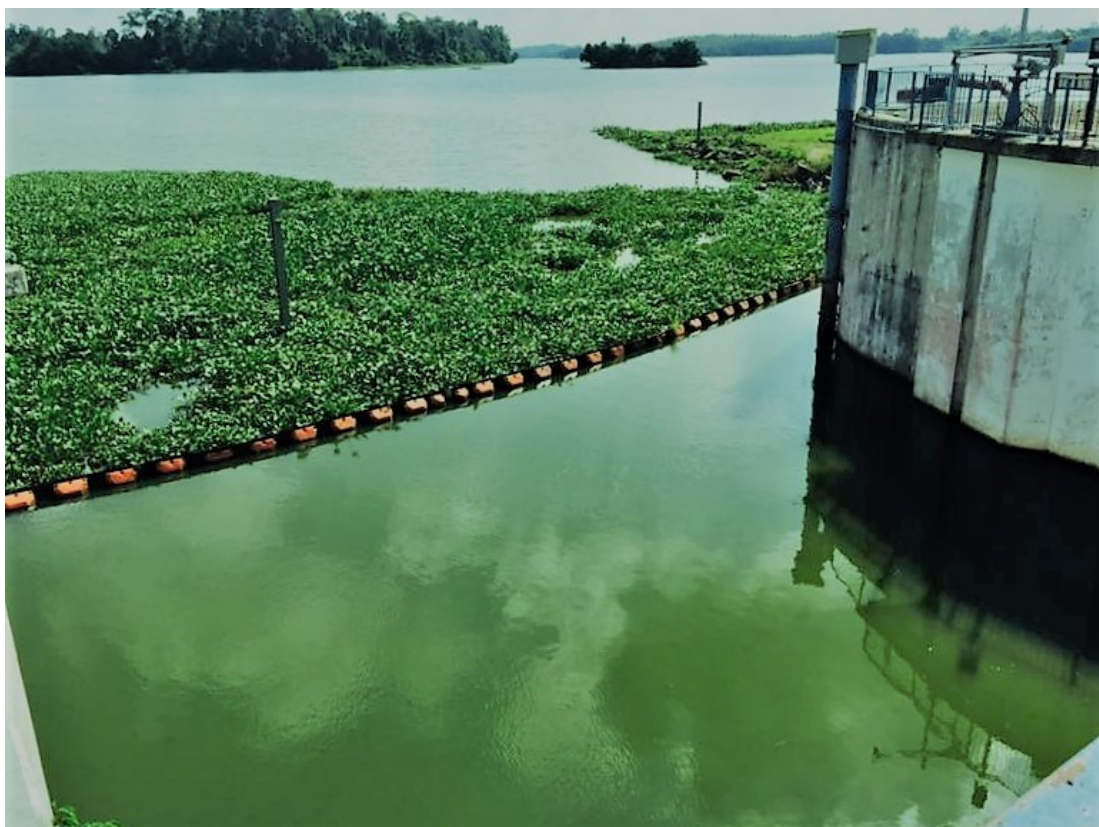
Figure 1.6 Polluted raw water from SBD. The dark green colour of the raw water shows a high content of microalgae which is difficult to be treated
