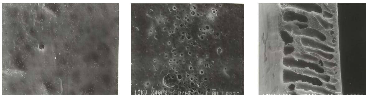
Figure 1. SEM Morphology of PSF-C4 Membrane Surface (a) upper, (b) lower, (c) cross section
