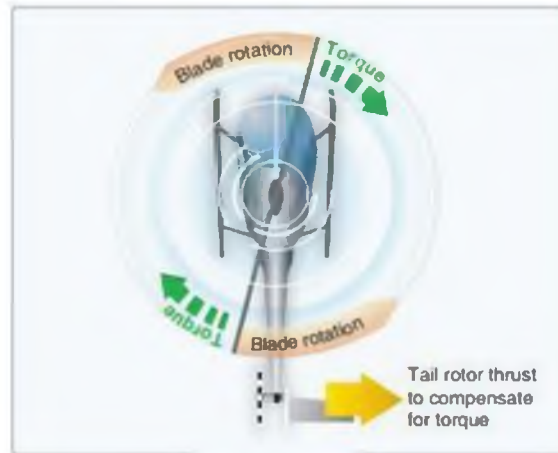
Figure 1 Anti-torque rotor produces thrust to oppose torque (FAA ,2012).
