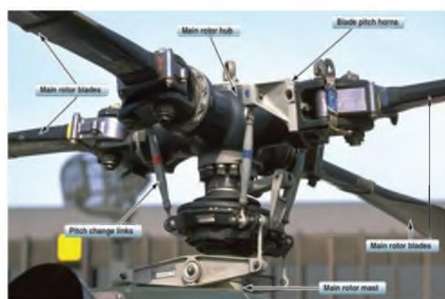
Figure 1.1 Main rotor hub assembly (FAA, 2012).
