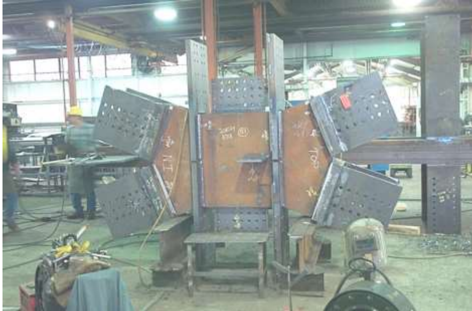
Figure 1.5 Prefabricated node. (source: http://buildcivil.wordpress.com/2013/ )
