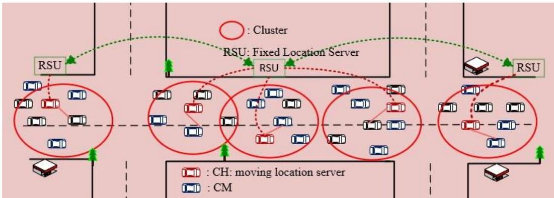
Figure 1.3 Clustering Based on Dynamic Clusters
